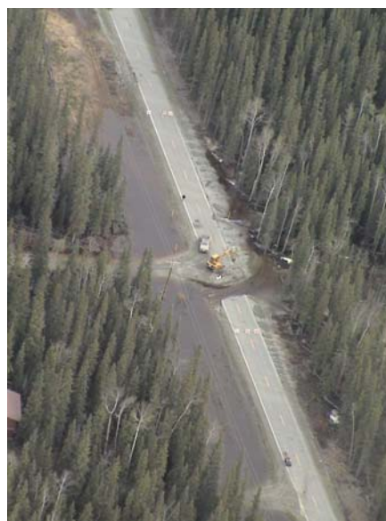
Photo 2: Aerial view of road breach to release flooding, May 2004.
